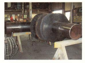
The design, fabrication and testing of a 20" ANSI 600 Y, 3 diameter radius, straight with a 90° lateral is ongoing.
