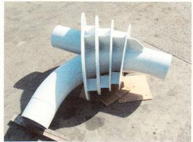
The pictures below are of two 8" ANSI 600 Y's with straight runs with one 90° and one 45° lateral. Both are 3 diameter radius bends for handling smart pigs.
