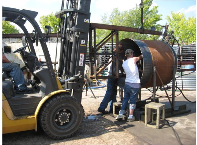
Forklift was used to install pig cup into test stand.
