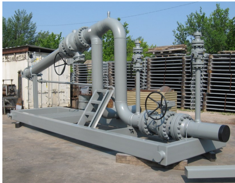
10" Sphere Receiver, skid mounted, with block valve and blow downs.
