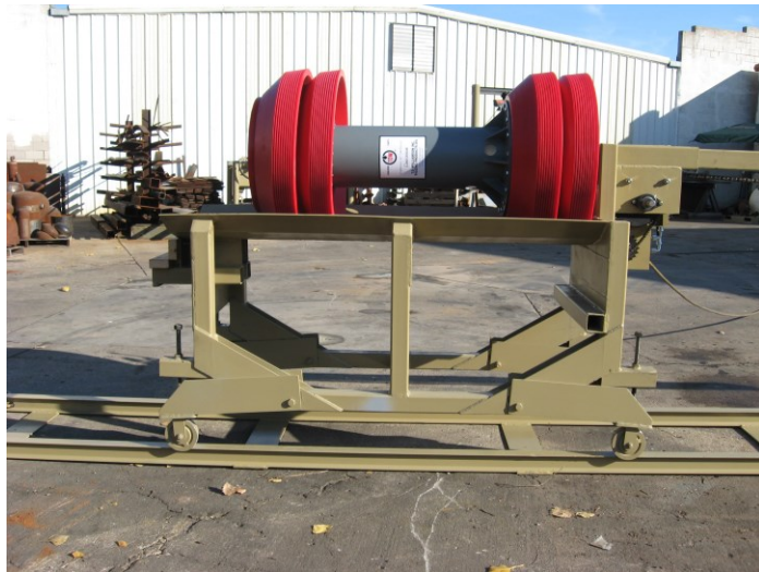
30" Pig Trap Launcher Tray with gas powered ram for advancing the pig to the barrel reducer
