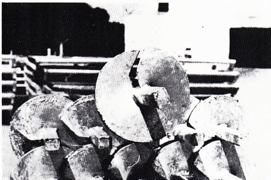
Newly developed beveled fluke on anchors for use in glacial soils (Fig. 5).
